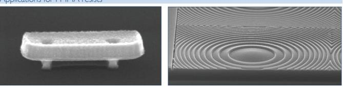
Fabrication of a PMMA bridge with AR-P 679.04 by exploiting Fresnel lenses with AR-P 671.09 the limited penetration depth at low acceleration voltage
