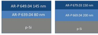
For these tests, the 2-layer systems were coated as shown to the left and tempered at 180 °C, 60 s, followed by irradiation with different doses (30 kV) and development (AR 600-60, IPA).
